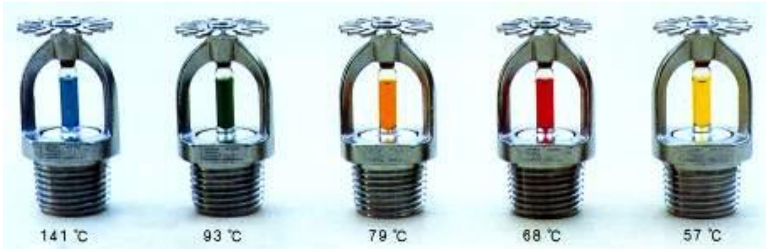
Automatic Fire Sprinkler Bulb Operating Temperatures
