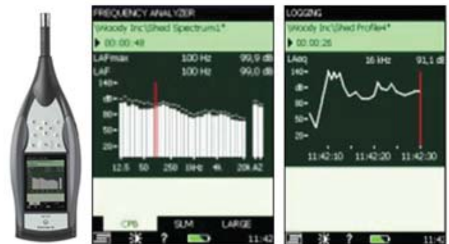
Fig. 2 Hand-held Analyzer Type 2250, module for frequency analysis and time module
