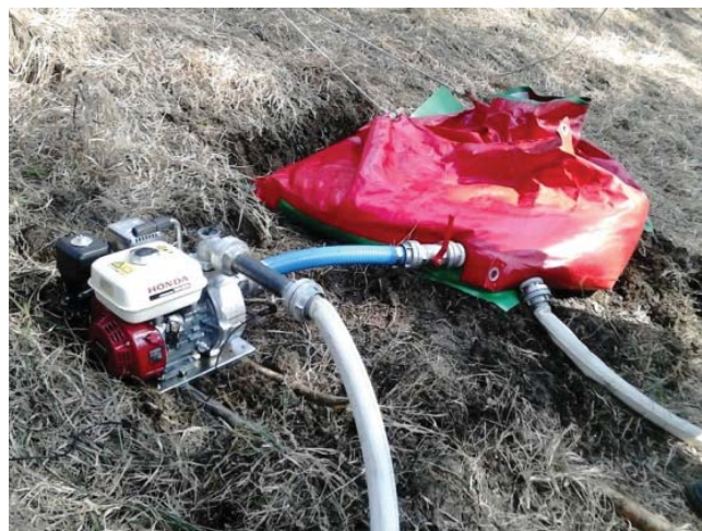
Fig. 1. The connecting of a pond with pump and hoses (photo: author)
