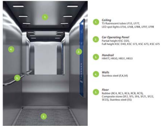
Fig. 5 Car interior options for firefighter elevators [7]
