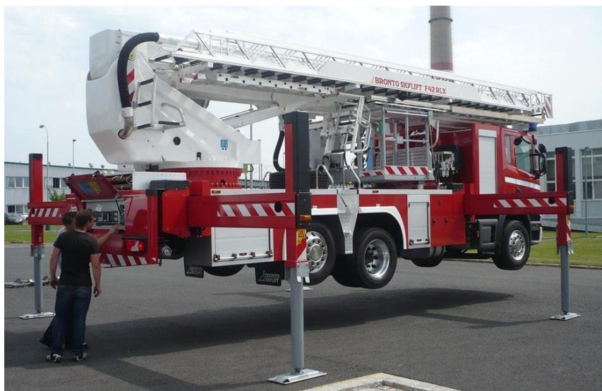
Obr. 31 Automobilová plošina Bronto Skylift F42 RLX [4]
